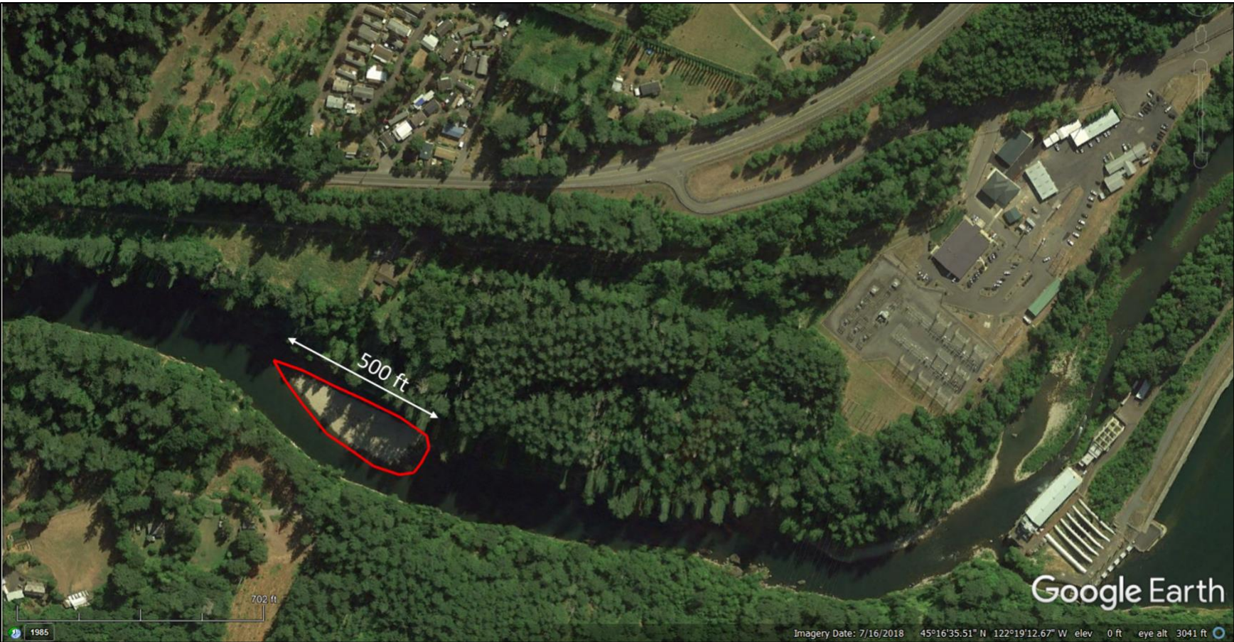
Figure 2. Aerial photograph of the proposed project site (enlargement of Figure 1). Red polygon surrounding the exposed bar is approximately 1.3 acres and is approximately 500 feet long. Habitat features would be constructed across the bar surface (which is commonly inundated) and along the shallow margins. The actual project area will be larger than the red polygon shown but depends on site bathymetry, i.e., the amount of available additional shallow water area where habitat features can be constructed.
